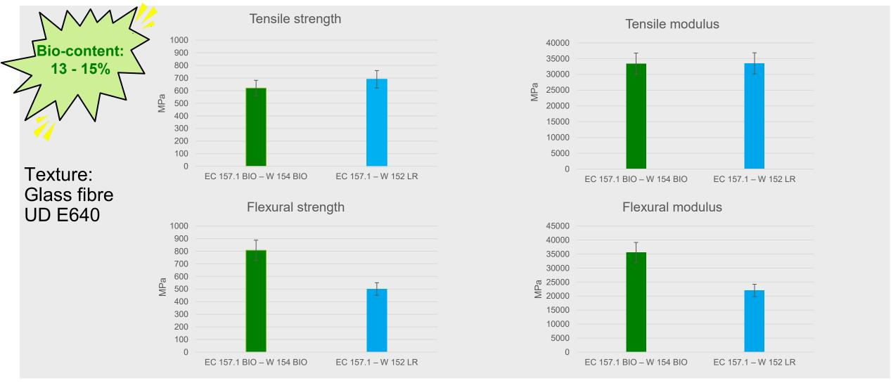
Mechanical properties of the bio-based systems are retained.
