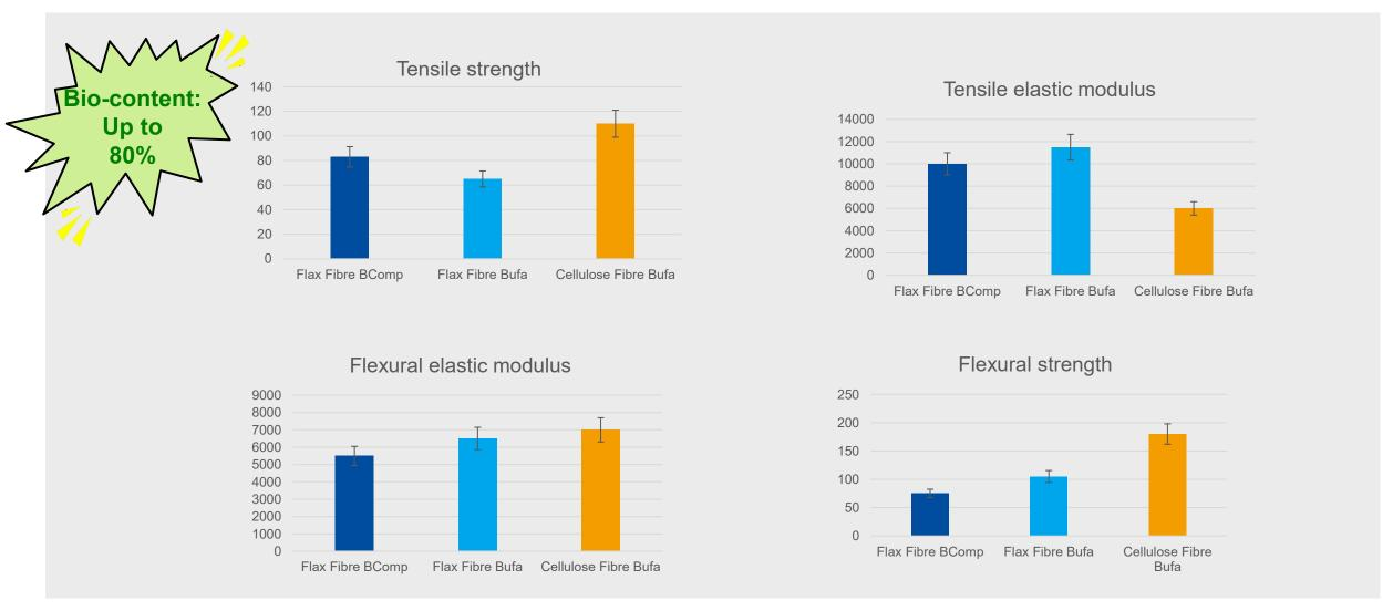
Cellulose is the most promising reinforcement fibre.
